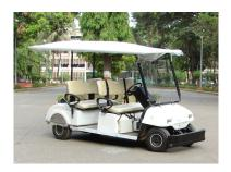
Intelligent autonomous transport vehicle is a fully autonomous vehicle used for transporting personals autonomously inside the campus. It is also used for advance research in mobile robotics. It is based on 4-seater electric-powered vehicle retrofitted with sensors and actuators to make it fully autonomous. It can maneuver autonomously around the campus based on the fixed waypoints as well as it can be driven manually.
